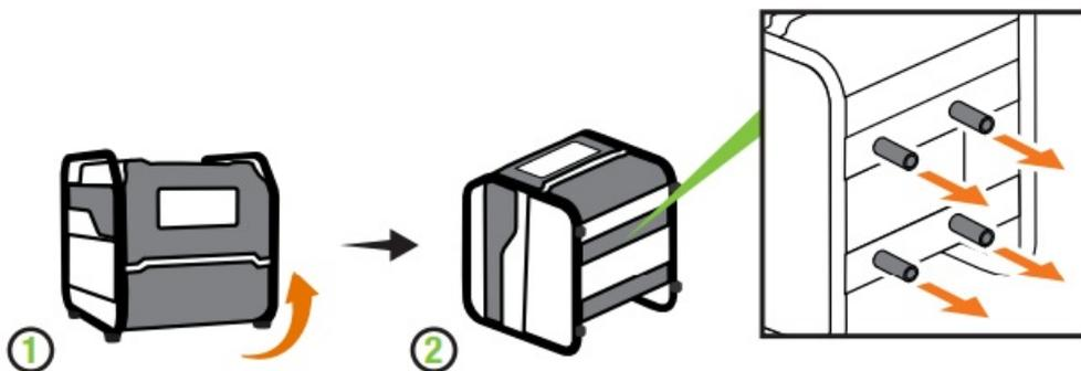
2. Attach wheel kit. Assembly > Install Wheel Kit
