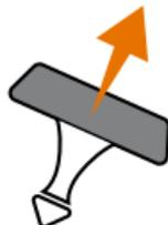
11. Move the choke lever to the "RUN" position.
