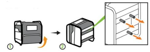
3. Attach wheel kit. Assembly > Install the Wheel Kit
