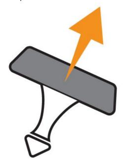
Pull the **recoil** to start the engine.
