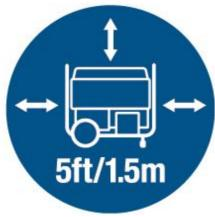
Keep all objects at least 5 feet (1.5 m) from the generator. The heat from the muffler and exhaust gas can ignite combustible materials.
