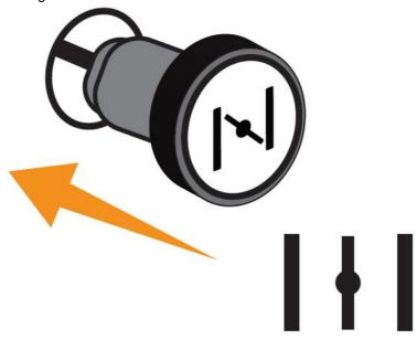
Push the **choke knob** into the "RUN" position.
