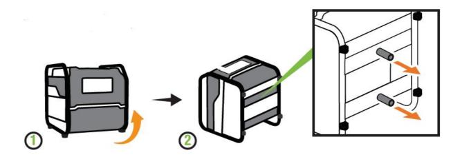
Remove shipping spacers. Assembly > Remove Shipping Support Spacers.
