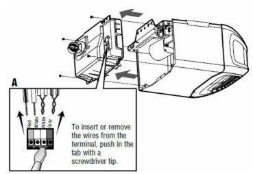
2. Unplug the wire harnesses from the receiver logic board. You may need needle-nosed pliers, to remove the harnesses.
