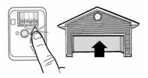
7. Press and release the DOWN Button. The door will travel to the programmed DOWN position. Programming is complete.
