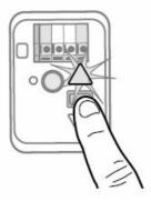
6. Press and release the UP Button. When the door travels to the programmed UP position, the DOWN button will begin to flash.
