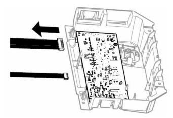
3. Remove the receiver logic board from the end panel by removing the 2 screws and releasing the 2 clips.
