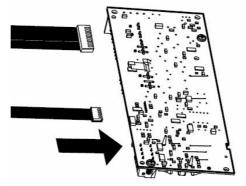
2. Insert the antenna wires through the holes in the end panel. Snap the receiver logic board into place on the end panel and fasten it with screws.
