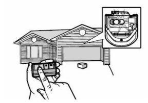
The garage door opener will not close from a remote control if the LED in either safety reversing sensor is off (alerting you to the fact that the sensor is misaligned or obstructed). If the garage door opener closes the door when the safety reversing sensor is obstructed (and the sensors are no more than 6 inches [15 cm] above the floor), call for a trained door systems technician.
