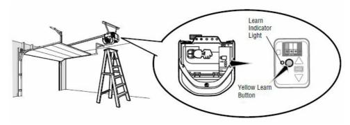
2. Within 30 seconds, press and hold the button on the remote control.
