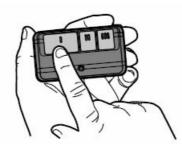
3. Release the button when the garage door opener light blinks. It has learned the code. If light bulbs are not installed, two clicks will be heard.
