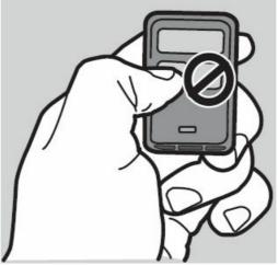
4. Press and release the Learn button on the garage door opener.
