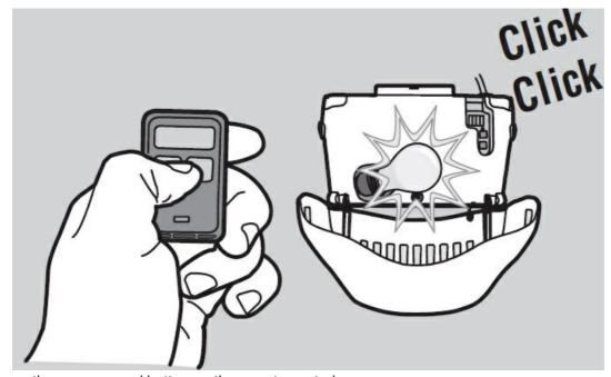
6. To test, press the programmed button on the remote control...
