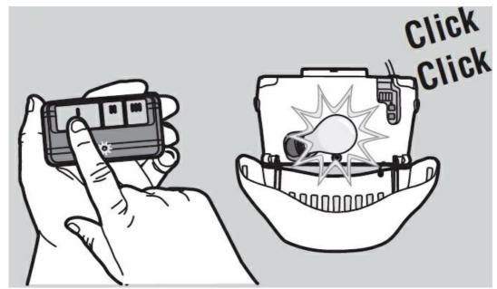
6. To test, press the programmed button on the remote control...
