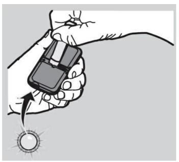
2. Press and release the remote control button you wish to use the number of times that corresponds with the garage door opener type:
