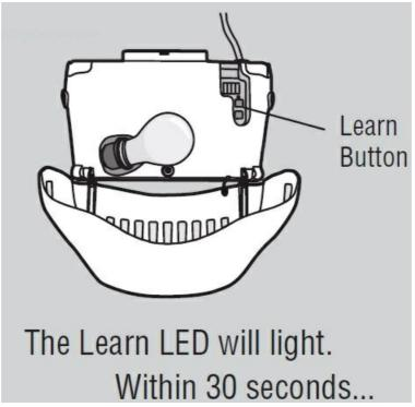
5. Press the remote control button programmed in step 2 until the garage door opener lights flash or two clicks are heard.
