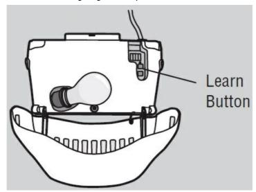
5. Press the remote control button programmed in step 2 until the garage door opener lights flash or two clicks are heard.
