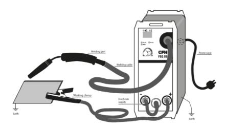
Supply cable hand torch hose package (-) | Ground terminal (+)
