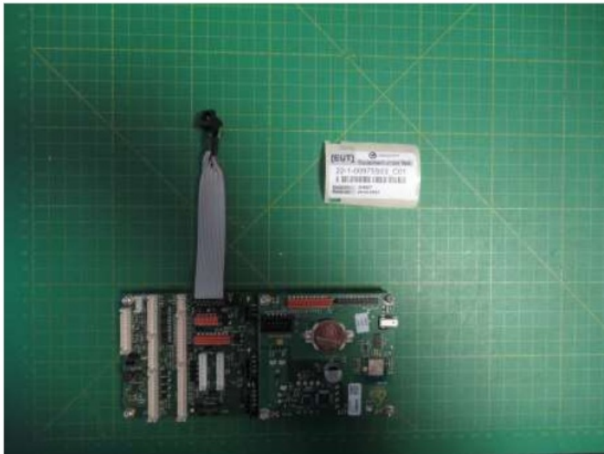
Photograph 2: EUT 2 – RF Board with RFID unit
