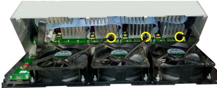
Figure 3: Disconnect the fan wires
