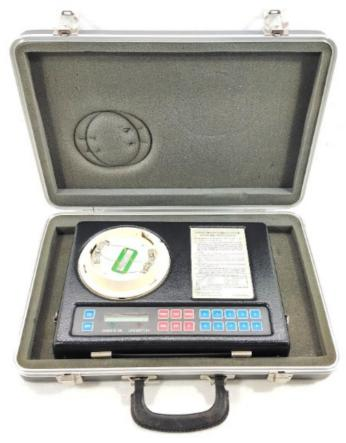
Sensor LINK Programmer and Tester For Intelligent Initiating Devices
