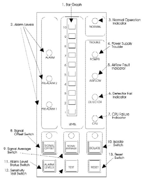
AnaLASER™ Control Card Front Panel Function Facilities
