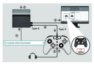
Ensure that 'Pro Controller Wired Communication' is turned on BEFORE connecting the controller and the Dock with the cable.
