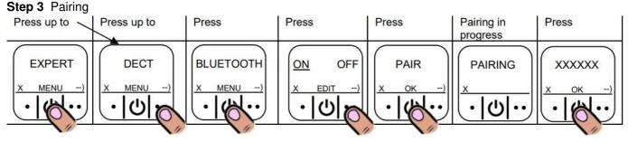
After confirming the pairing code, the name of the other Bluetooth device is displayed. The devices are now connected via Bluetooth. If the pairing process takes longer than 1 minute, the CT-DECT Multi M7 interrupts the process with the message "Time Out".
