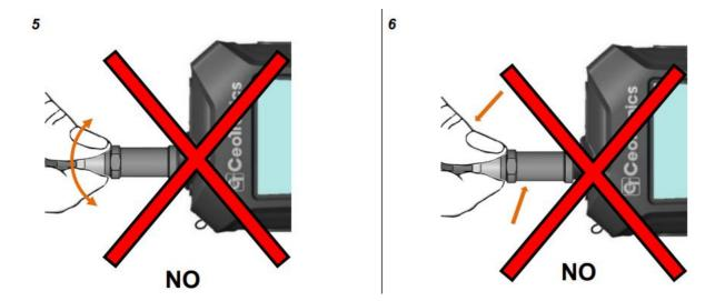
The locked connector must neither be twisted (Figure 5) nor kinked (Figure 6). Improper handling can damage the connector.
