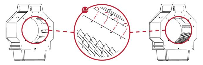
A. Reach inside the machine and install the Blade Sheet by gently placing the sheet on the metal tabs until all holes are resting evenly on metal tabs on both sides of the machine
