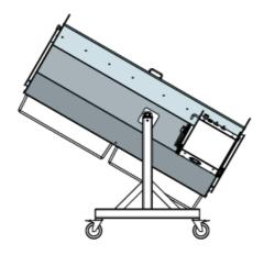
facing posi-tion, replace Plunger. Load dried, prepped, untrimmed plant material into the Tumbler. For best efficiency, fill Tumbler 40-60% full and run batches of similar material.
