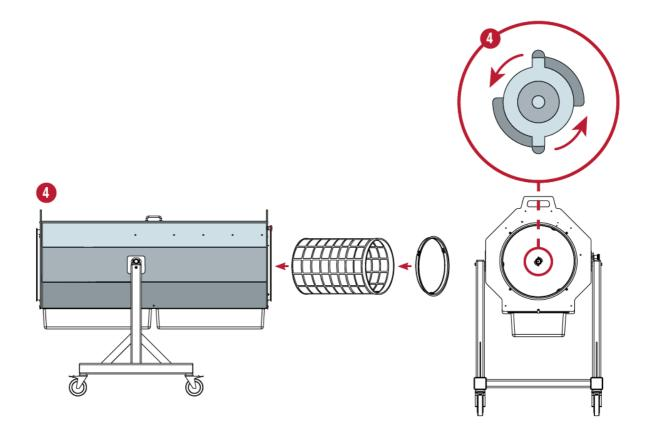
With motor off, power cord unplugged, and machine in a vertical position, slide Filter Screen gently into machine. Rotate Tumbler counter-clockwise to lock.
