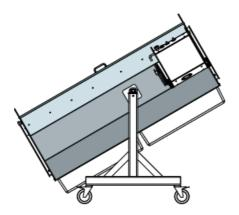
Once desired trim is accomplished, remove Trim Tray & Tumbler Lid, position separate container (not included) to capture processed material, pull out Plunger and pivot drum to a downward facing position. Processed material will be deposited in container when correctly positioned.
