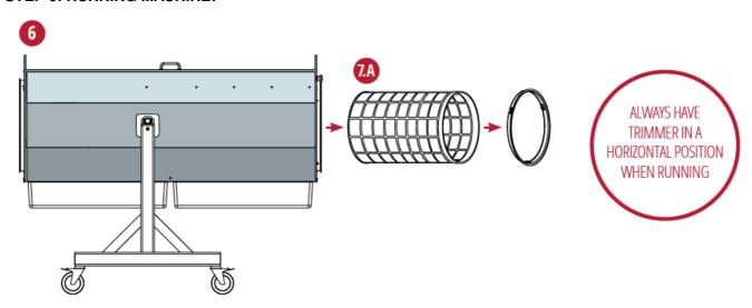
Rotate the Trimmer into a horizontal position and turn machine ON. Run materials for up to 10 minutes.
