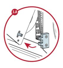
**A.** Release side drive by removing the 2 locking pins.
