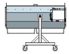
Re-apply clear Tumbler Lid. Pull out Plunger and pivot Drum into a horizontal position. Tighten Blade Sheet as required. Turn ma-chine ON and allow to run for 1-15 minutes. Check material every 2-5 minutes. For a closer trim, continue running the DBT Model 4 until desired trim is accomplished.
