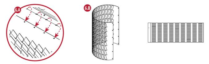
• A. Reach inside the machine and remove the Blade Sheet by gently lifting the Blade Sheet off of the
