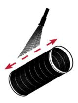
Clean the length of the tumbler of all debris using hot pressurized water.
