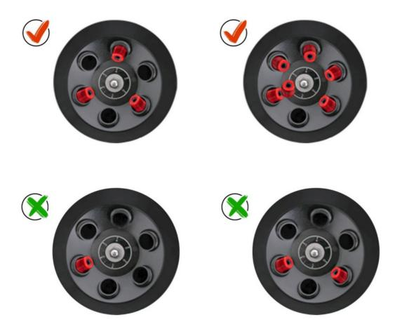
• f. Graphic presentation about the correct placement of centrifuge tubes (8 holes).
