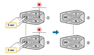
After few seconds the units will be paired and they will start the intercom communication. The light on both units will flash blue twice.
