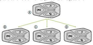
The pairing is only necessary the first time, then the control units will automatically recognize each other.
