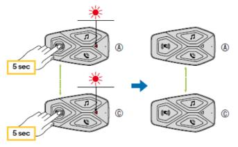
3. Repeat the procedure again, pressing the centre button (intercom) of the two units A and D for 5 seconds until you hear the voice prompt "Intercom pairing".
