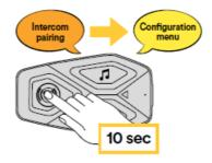
With U-COM 3 on, enter the configuration menu by pressing the power key for 10 seconds. Be careful not to release the button before the LED turns blue, you will hear the message confirming activation of the configuration menu.
