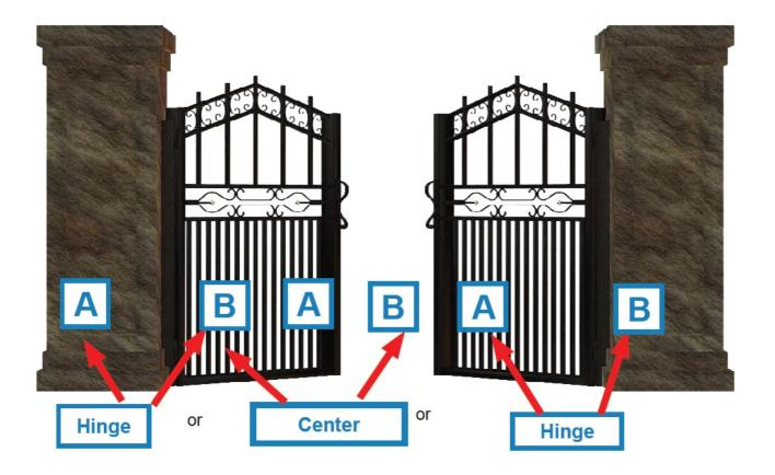
Place the Mag Switch anywhere you can pull A and B at least 2 inches away from each other when the gate is open, and where you can pull A and B 1.5 inches apart when the gate is open.
