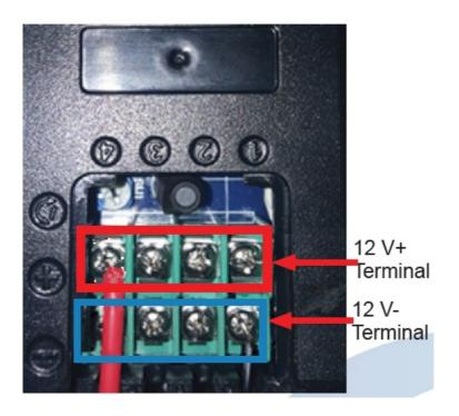
Interface Circuit Board (Oriented the same as the Watchman install)
