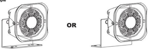
The bracket may be mounted in any direction as long as the speaker "TOP" marking is oriented upwards for proper drainage.
