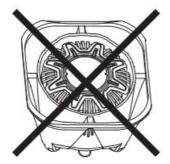
Do not mount the speaker with the bell opening facing upward.
