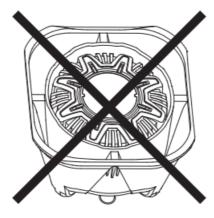
Do not mount the speaker with the bell opening facing upward.
