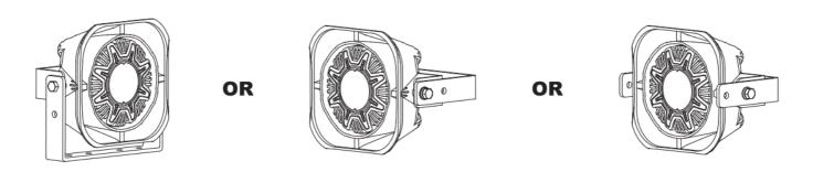
The bracket may be mounted in any direction as long as the speaker "TOP" marking i s oriented upwards for proper drainage.
