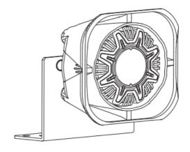
The bracket may be mounted in any direction as long as the speaker "TOP" marking is oriented upwards for proper drainage.
