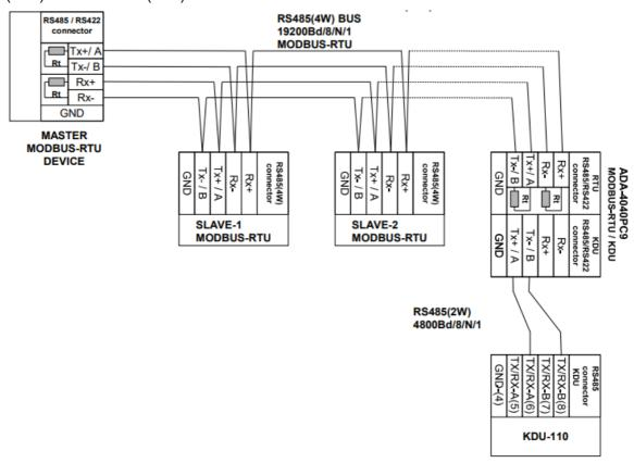
Example connection of the KDU-110 device by the use of ADA-4040PC9 to RS485(4W) 4-wire bus.
