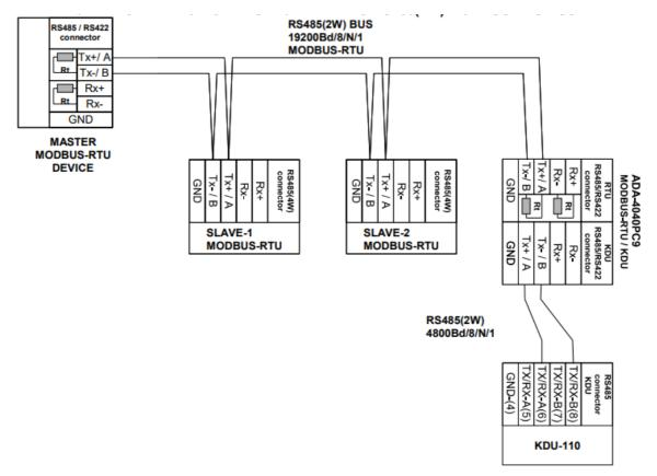
Example connection of KDU-110 device by the use of ADA-1040PC9 to RS485(2W) 2-wire bus.
