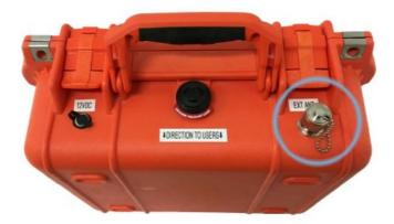
To received a mobile signal an external antenna that supports all cellular bands must be connected to the antenna port.
