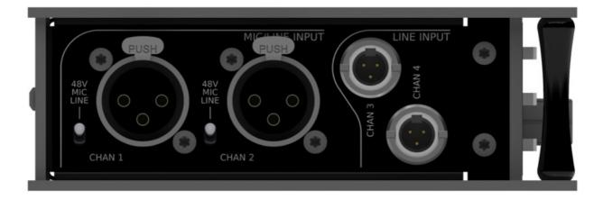
If you wish to send digital signals to the DNS 4, use the AES 3 inputs. The input selection is set using channel button 1 in the Setup page. Press setup twice to
