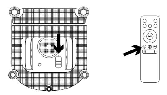
Press Start/Pause and Clean keys on the remote control to check the driving wheels, if there is any dust, press pause and clean the dust.
