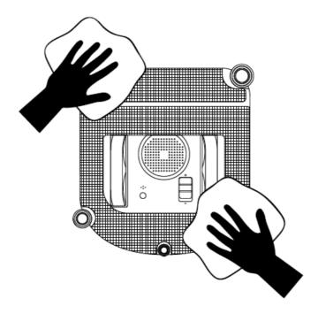
**Driving treads:** Before cleaning the wheels, move the power switch to the "-" position. Then wait 8 seconds until it stops suctioning and starts beeping. Then press " " key on the remote control and start cleaning the driving wheels.
