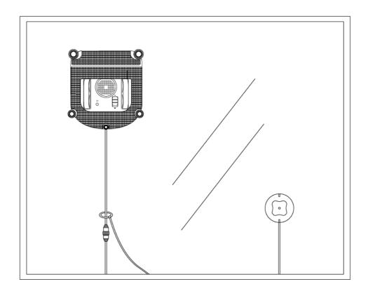
Wipe the surface of the safety pod's suction cup clean with the provided finishing cloth.
