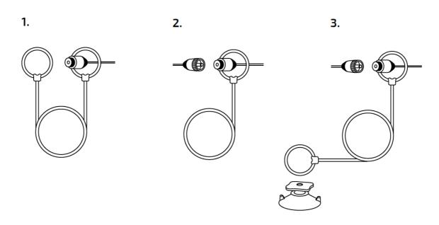
If the length of the power cord restricts the robot's movement, an extension cord of the robot can be used. Disconnect End A and End B, and connect them with both Ends of the extension cord respectively and tighten. Only one extension cord can be used with the robot.
