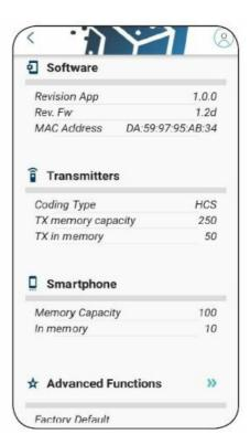
Set or change the name of the receiver. Set the relay operating mode: PULSE, LATCH, TIMED. In Timed mode, it is possible to set the relay release time from 1 sec. to 23h: 59m: 59s. Collection of all the information regarding the receiver (passwords, software version, coding type etc..)
