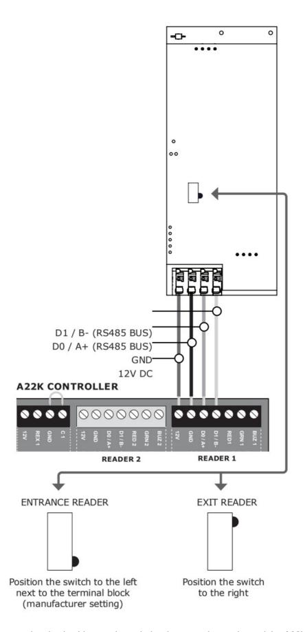
It is recommended to use twisted pair wiring as shown below between the reader and the A22K ATRIUM controller.
