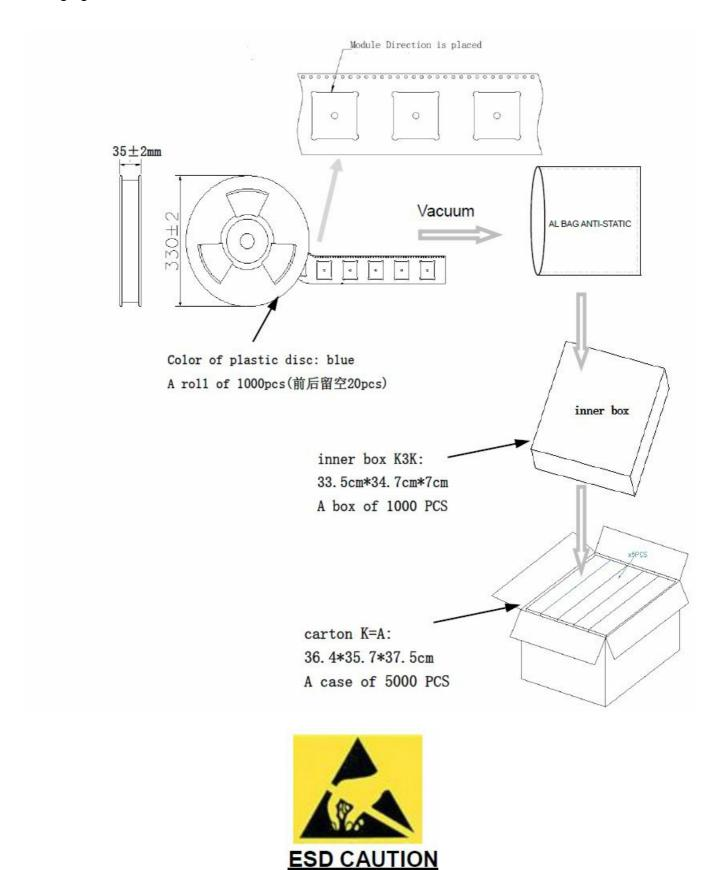
The 6986850 6986850-00 module is an ESD (electrostatic discharge) sensitive device and may be damaged with ESD or spike voltage. Although the 6986850 -00 module is with built built-in ESD protection circuitry, please handle with care to avoid the permanent malfunction or the performance degradation.
