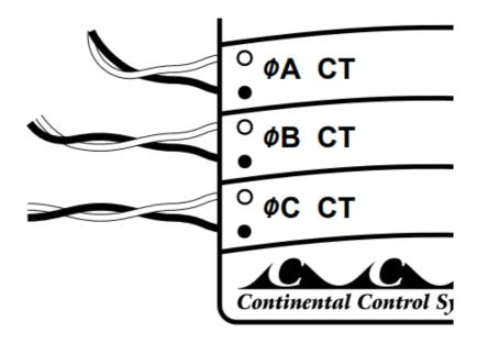
**Note:** Be careful to match the CT to the voltage phases being measured. Make sure the  $\varnothing A$  CT is measuring the current on the  $\varnothing A$  conductor, and the same for phases B and C. Use colored labels or tape to identify the wires.
