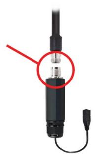
2. Once the antenna is securely screwed onto the CC DX Mile, use the supplied coaxial seal to completely cover the connection.
