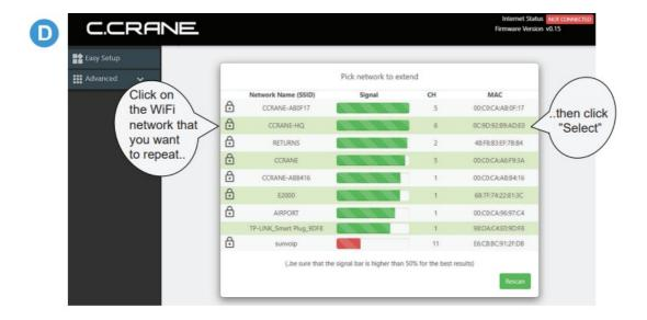
NOTE: For best performance, your signal should be higher than 50%. For a better signal, try adjusting the orientation and placement of the USB antenna – then click "Rescan" to see if the signal is higher.
