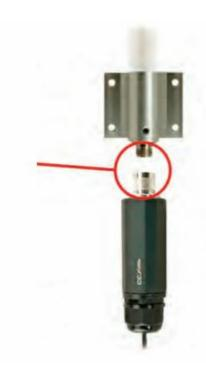
Before connecting the CC X Mile to the antenna, coat the threads of the antenna with the supplieds silicone grease. This will help protect the threads from rust and water incursion.
