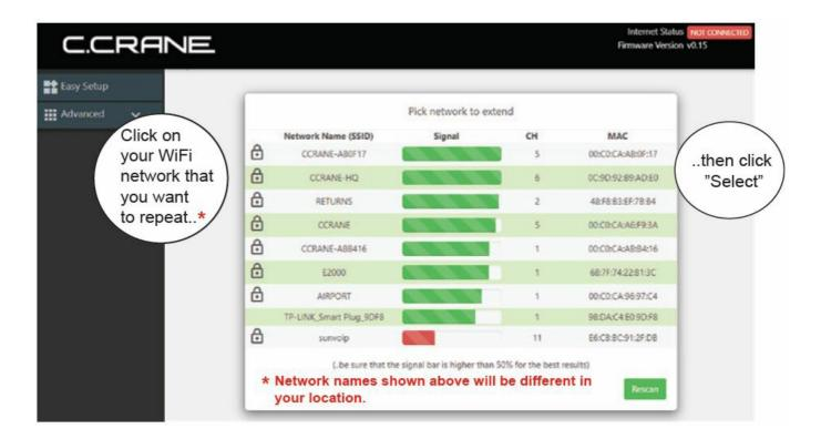
**NOTE:** For best performance, your signal should be higher than 50%. For a better signal, try adjusting the orientation and placement of the USB antenna – then click "Rescan" to see if the signal is higher.
