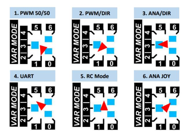
When power on or changing mode. The Run LED in the PCB will blinking a X sequence number to confirm witch mode are configured. X = 1 (PWM 50/50), X=2 (PWM/DIR),..., X=6 (ANA/JOY)
