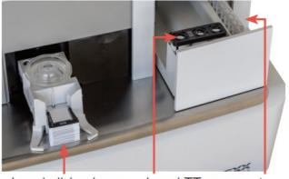
Load slides here Load TT<sub>4</sub> reagent and tips here
