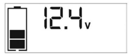
The bars on the Battery Status Icon represent the charge level of the unit's internal battery. The bars on the Battery Status Icon will change from empty to solid (bottom to top) repeatedly to indicate the unit is charging. The backlight will turn on for 10 seconds (only).
