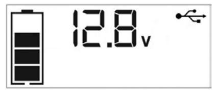
The Battery Status Icon and Battery Voltage Indicator will light solid, as well as the USB Icon, indicating the USB ports are ready to use.
