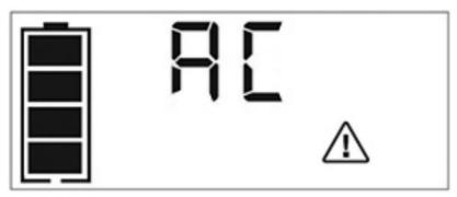
The Digital Display will show "AC"; the FULL Battery Status Icon and Fault Icon on the LCD Screen will flash.
