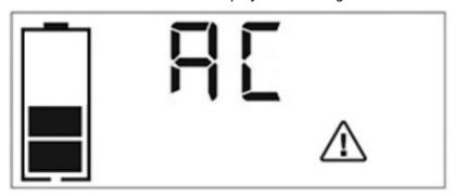
The Battery Status Icon will light solid; the "AC" on the Digital Display and the Fault Icon on the LCD Screen will flash.
