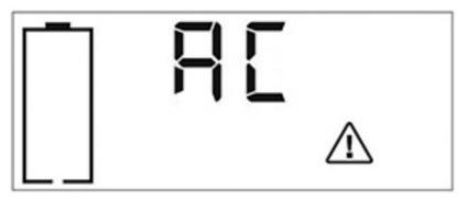
The Digital Display will show "AC"; the EMPTY Battery Status Icon and Fault Icon on the LCD Screen will flash for 10 seconds before the unit automatic shut down.
