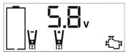
The Battery Status Icon, the Battery Voltage Indicator, Clamp Icons and the "+" and "-" signs light solid to indicate the unit is jump-starting.
