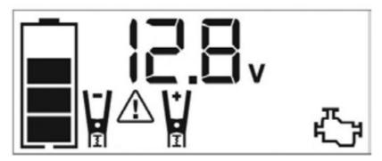
Turn off the Jump Starter Power Switch; connect the clamps to the battery, making sure the clamps are connected with correct polarity; then turn the Jump Starter Power Switch back on.
