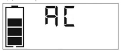
The Battery Status Icon lights solid and the Digital Display shows ""AC", indicating the AC outlet is ready to use.
