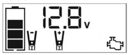
The Battery Status icon, Battery Voltage Indicator, Clamp Icons and the "+" and "" signs light solid. The jump starter icon will flash to indicate the clamps are properly connected.
