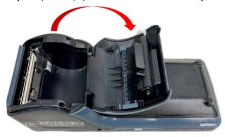
• Step 3. Insert the paper roll into paper roll slot and close the paper roll cover counter clock wisely.
