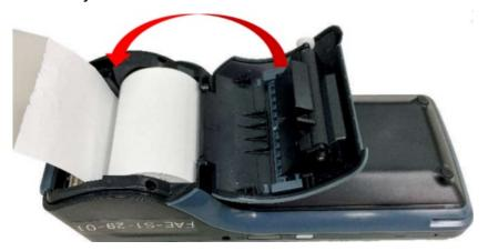
• Step 4. When closing the paper roll cover, make sure some portion of paper is out of the printer.
