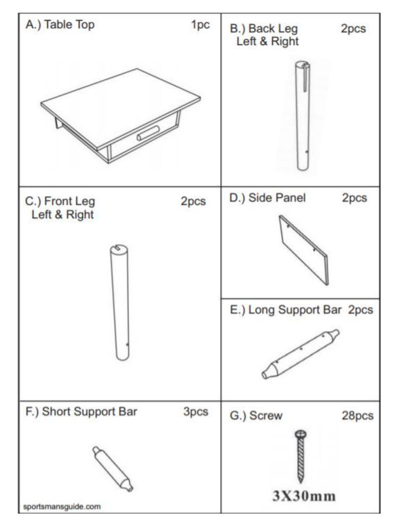
Attach the three Short Support Bars (F) into the Long Support Bars (E) and secure both sides in place using Six Screws (G).
