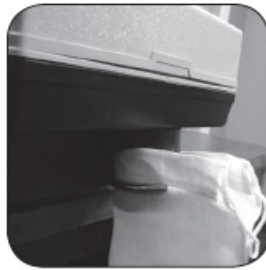
Proper attachment of a coin bag.
