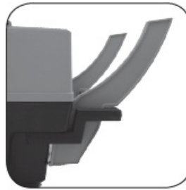
Correct position for hopper cover brackets
