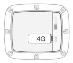
Step 4: Install the top cap, tighten the screws and insert the top screw cover
