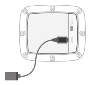
Step 4: Pass the USB cable through the USB hole, install the top cap, install the silicone plug-in USB hole, and then connect the USB cellular modem to USB cable
