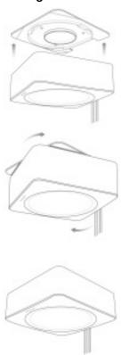
**IMPORTANT:** For best range results, we recommend mounting the S2000 on the ceiling in an unobstructed location.
