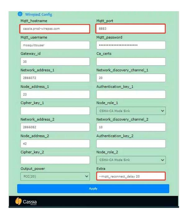
Figure 10, Gateway Configuration
