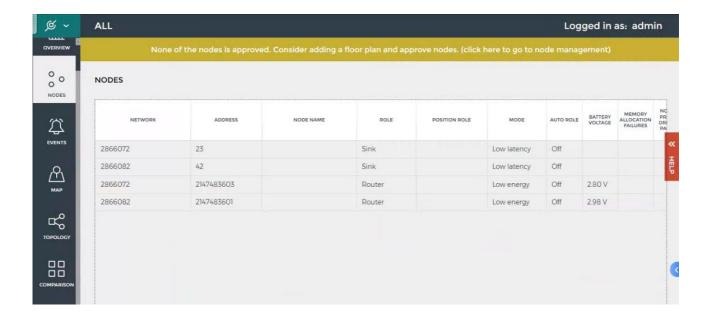
Figure 4, WNT Tool, Nodes view
