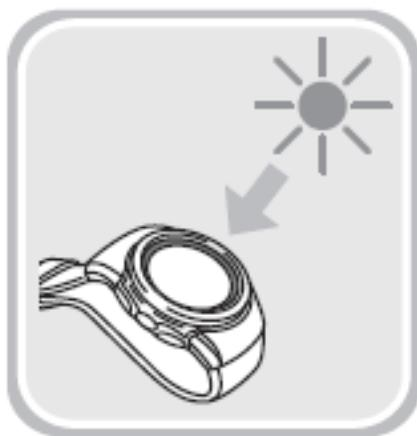
When wearing the watch, try to keep your clothing from blocking its face (solar panel). Charging efficiency is reduced significantly even if the face is blocked only partially
