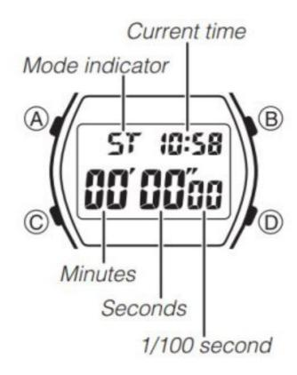
The stopwatch lets you measure elapsed time, split times, and two fi dishes. The range of the stopwatch is 23 hours, 59 minutes, 59 seconds.
