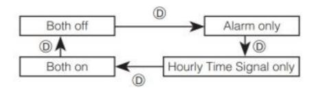
• The alarm on indicator and the Hourly Time Signal on indicator is shown on the display in all modes while these functions are turned on.
