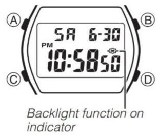
In the Timekeeping Mode, hold down D for about two seconds to switch the backlight function on and off. When you switch the backlight function on, an indicator appears on the display as shown.
