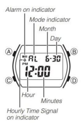
The multi-function alarm lets you specify the hour, minutes, month, and day for the alarm (page E-14). When the alarm is on, the alarm sounds for 20 seconds at the preset time. When the Hourly Time Signal is on, the watch beeps every hour on the hour.
