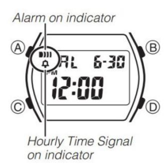
Press D while in the Alarm Mode to change the status of an alarm and Hourly Time Signal in the sequence shown below.
