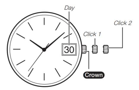
Some water-resistant models (10BAR, 20BAR) have a screw-in crown. When you need to perform a crown operation, rotate it towards you to unscrew it. Then pull the crown out. Avoid applying undue force when pulling. The watch loses its water resistance while the crown is unscrewed. After performing a crown operation, fully screw the crown back in.
