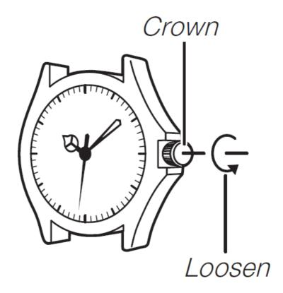
Some water-resistant models (100 meters, 200 meters) have a screw-in rown. When you need to perform a crown operation, rotate it towards you to unscrew it. Then pull the crown out. Avoid applying undue force when pulling. The watch loses its water resistance while the crown is unscrewed. After performing a crown operation, fully srew the crown back in.
