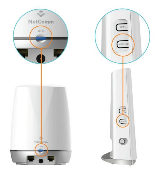
Network Ports for non-wireless devices. Up to two devices may be connected.
