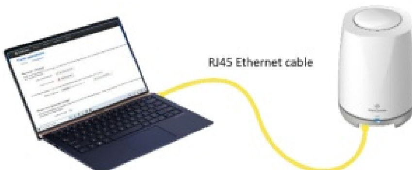
Figure 10 – Ethernet cable connecting PC with CloudMesh Satellite
