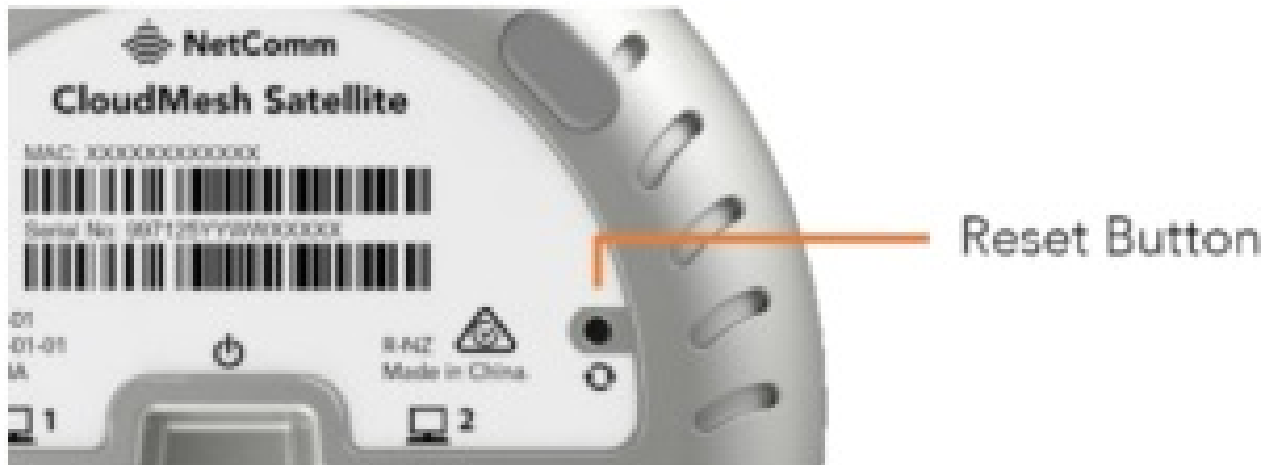
Figure 17 – Location of reset button on bottom
