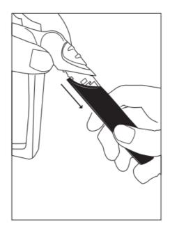
2. Insert 1 AAA battery in the correct polarity, then replace battery handle.
