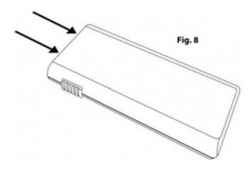
To protect lens from scratching, push lens housing back into base when not in use (Fig. 8).
