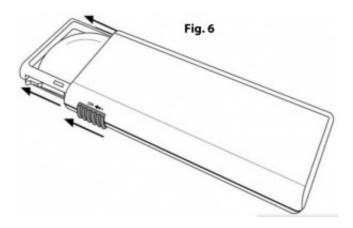
Slide switch located on side of base forward to extend lens (Fig. 6).
