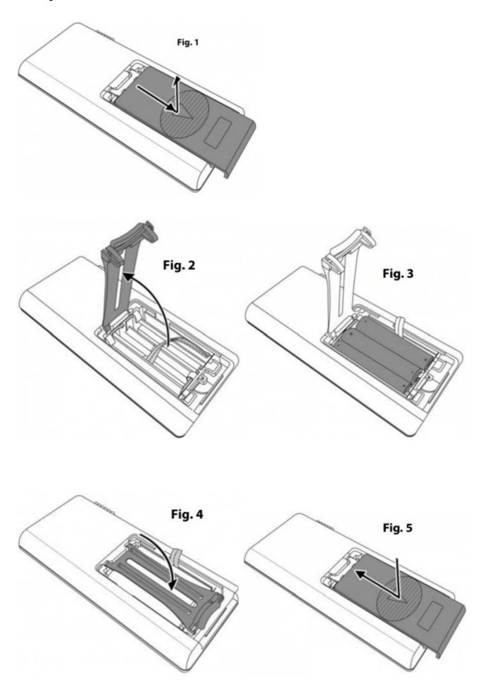
Make sure lens is positioned inside of protective case. Slide battery door down and remove (Fig. 1). Lift gray plastic brace up (Fig. 2). Insert 3 AAA batteries according to the polarity indicators marked on the inside of battery
