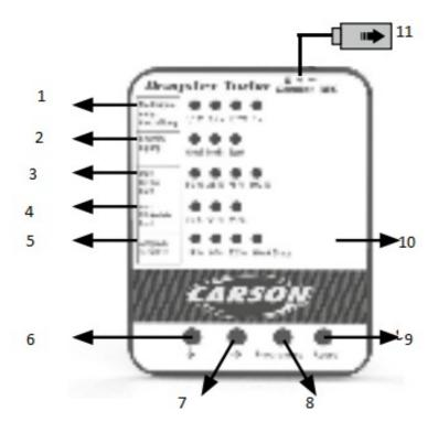
1. Low Voltage Cut-Off: The function is mainly to prevent the lithium battery pack from over discharging. When using lithium battery pack, please set the suitable value for low-voltage protection as your like.
