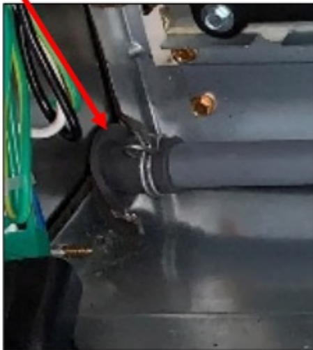
Fig. 4 Formed Grommet Secured to Z-Pipe
