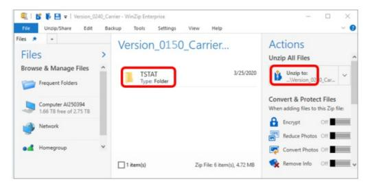
• Choose the USB-C drive as the location to which to extract the folder from the zip file. This will create a new TSTAT folder or over-write the existing TSTAT folder and any files contained within it. Click Unzip.
