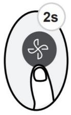
Keep pressing Fan button for more than 2 seconds to activate/disable Silence function(some units).
