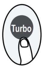
When you select Boost feature in COOL mode, the unit will blow cool air with strongest wind setting to jump-start the cooling process.
