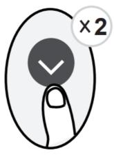
The unit will operate at high fan speed (while compressor on) with temperature automatically set to 8 C/46 F. **Note:** This function is for heat pump air conditioner only.
